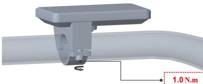
② Open the holder ring/rubber spacer of the keypad and fix it on the handlebar, adjust it to a proper facing angle. Use a M3 Hex Wrench to fix and tighten the screws. Standard fixing torque: **1N·m**.
